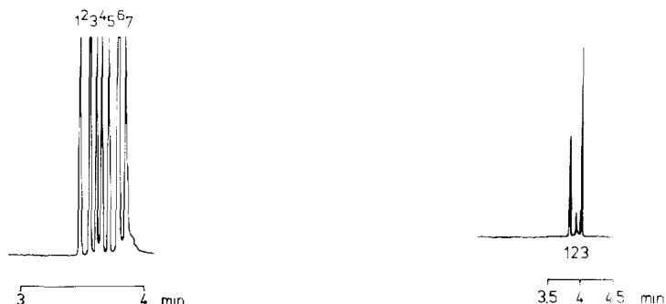
Fig. 3. Separation of tramadol, internal standard and five metabolites. Peaks: 1 = tramadol, 2 = M2; 3 = M3; 4 = internal standard; 5 = M1; 6 = M5; 7 = M4.
